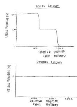
Electric Potential Height Maps show causes to the differences between series and parallel circuits
